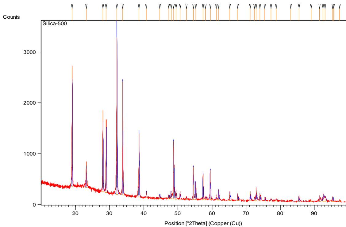
**Fig-2 ( X-RD of Silica 500 sample)**
