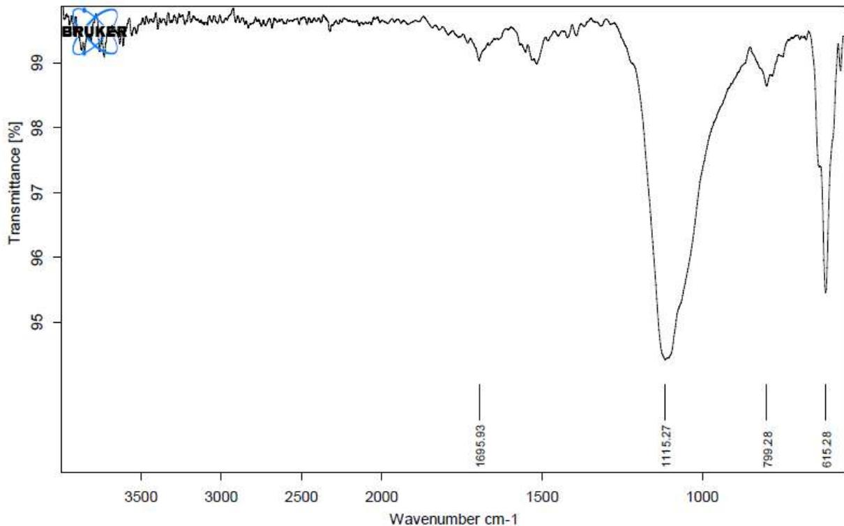
**Fig-5 FTIR of Silica700**
