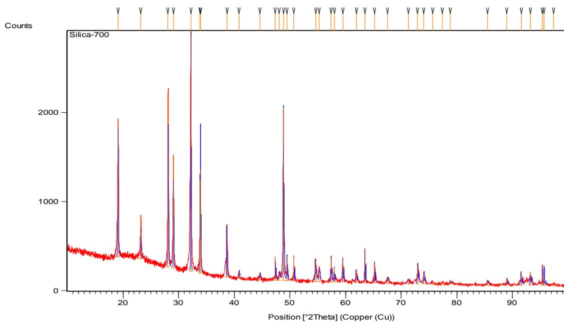
**Fig-3 (X-RD of silica 700 sample)**
