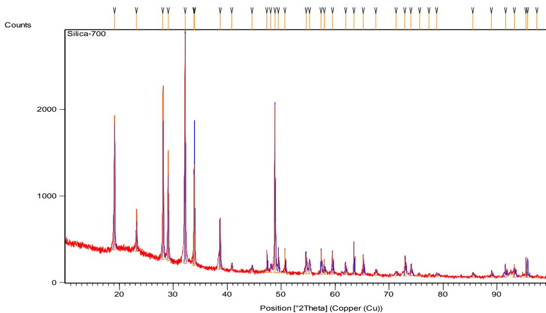
**Fig-3 (X-RD of silica 700 sample)**
