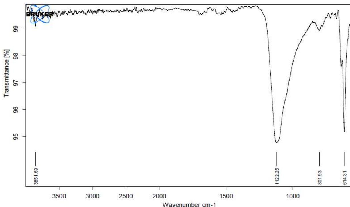
Fig-4 FTIR of Silica 500
